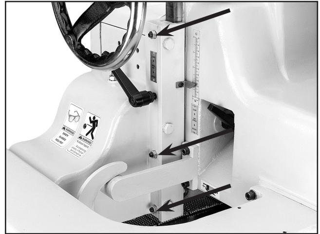
Figure 33. Gib adjustment setscrews.
